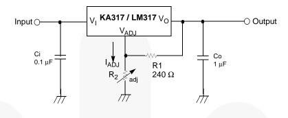
$V_0 = 1.25 V (1 + R_2 / R_1) + I_{ADJ}R_2$
