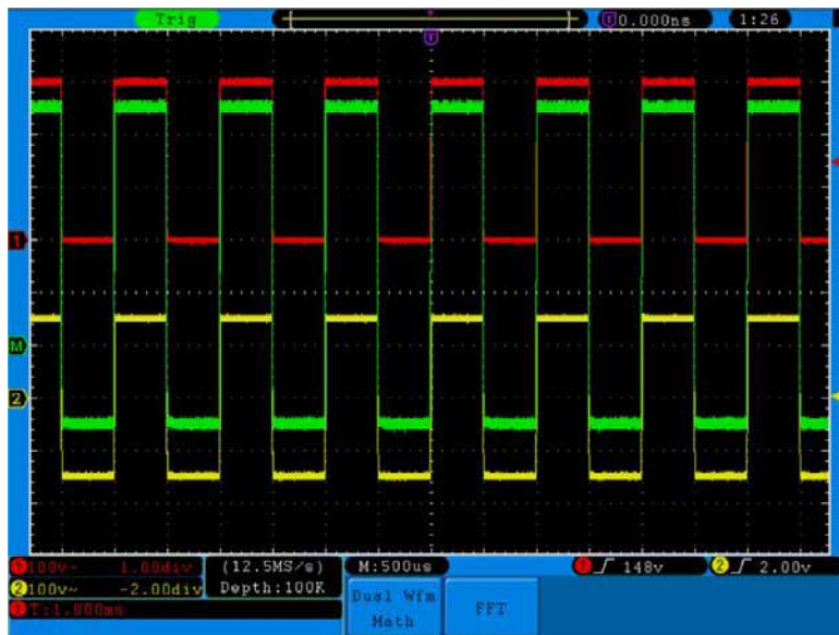
Fig. 19 Waveform resulted from CH1 +CH2 Mathematical Manipulation
