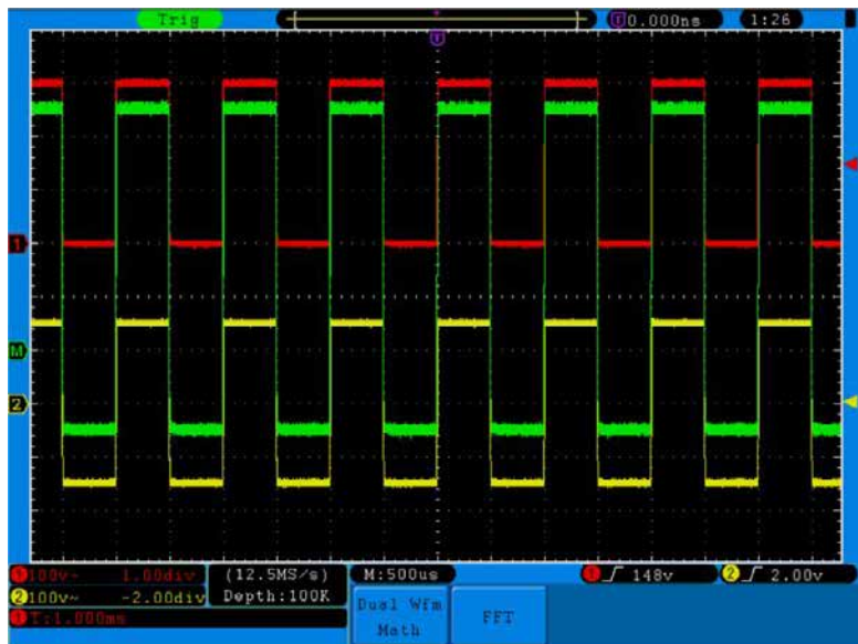
Fig. 19 Waveform resulted from CH1 +CH2
