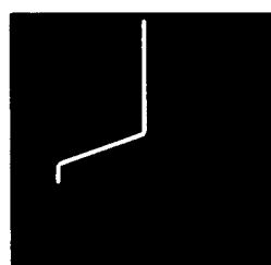
B-E paralleled by 680Ω
