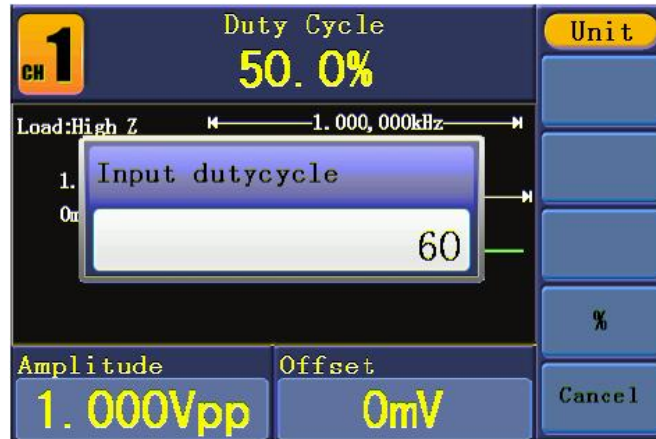
Figure 0-8: Set the Duty cycle of Square signal
